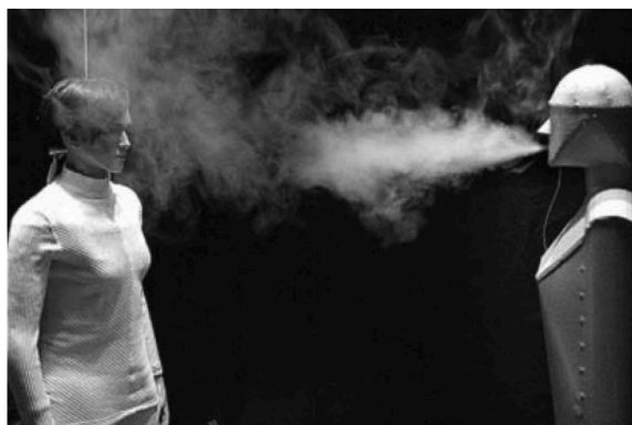
Fig. 2b. Smoke visualisation of exhalation flow from mouth of mannequin on the right. The breathing zone of mannequin the left mannequin is obviously penetrated despite a distance of 1.2 M [14].
